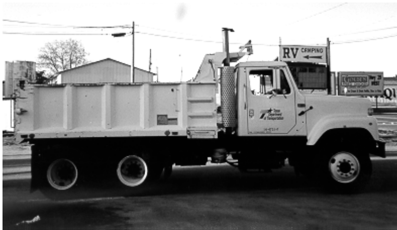
Figure 4.6 TxDOT loading vehicle
